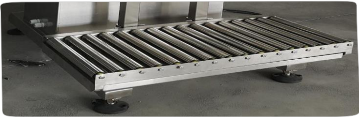
Out feed Roller conveyor
